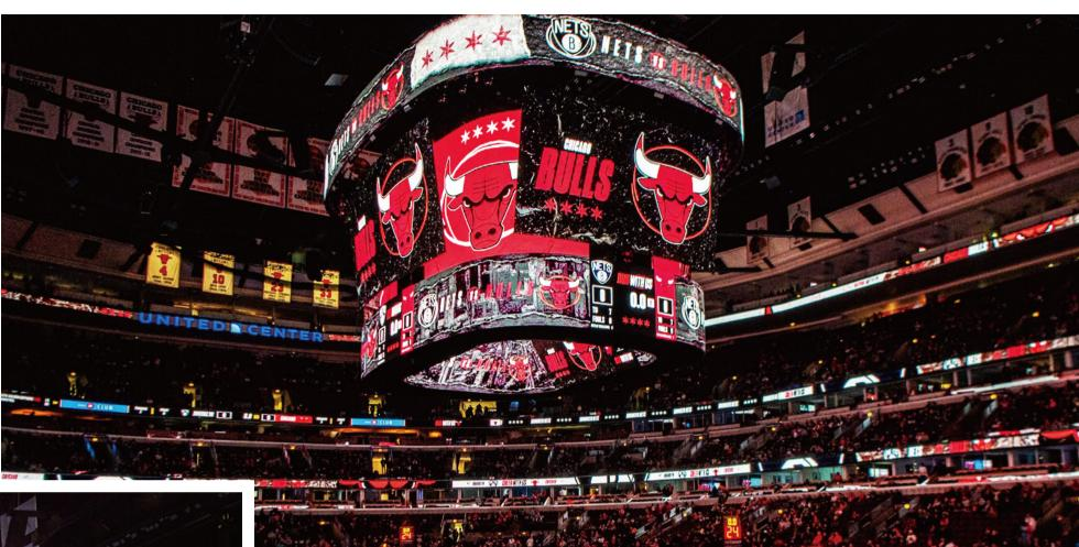
The state-of-the-art scoreboard, with a 4mm pixel pitch, is around about 8,600ft<sup>2</sup>(800m<sup>2</sup>) and has a 4K resolution, making it the largest and clearest center-hung display of its kind in NBA and NHL arenas. It employed YAHAM's CH series, which has a lightweight of just 18kg/m<sup>2</sup>, significantly reducing the load capability of the center and ensuring the smooth operation of the kinetic drop-down technology.
